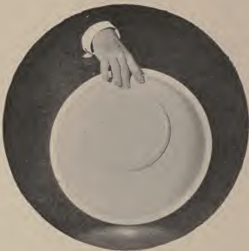
Starting the spin of a basin. Second finger and thumb grasping the rim.
